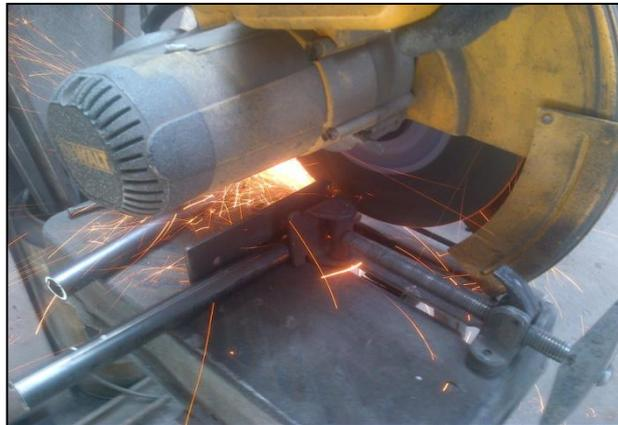
**Figura 6.2: Corte de tubo ASTM A-500 Grado B.**
