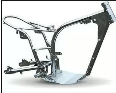
**Figura 2.5: Bastidor multi-tubular cuna simple.**
