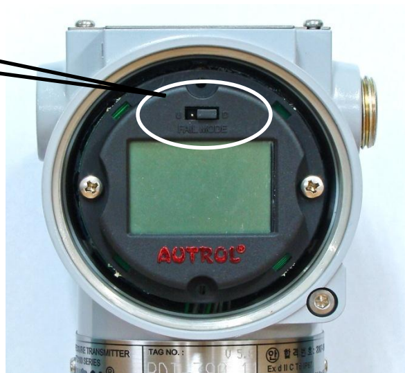
Figure 3-2 Fail Mode Selection Jumper Switch of LCD Module
