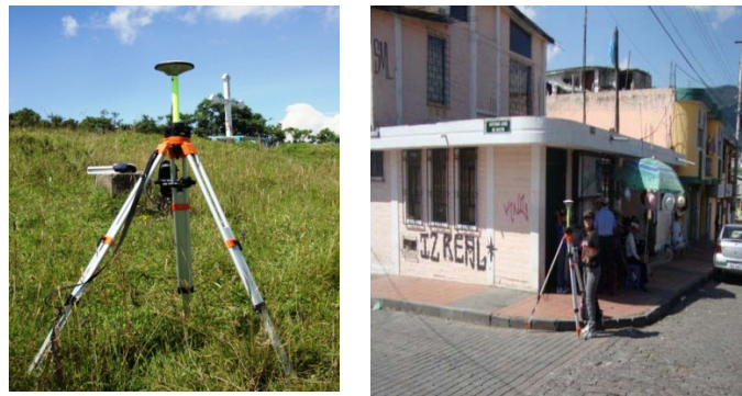
Figura 8: Receptor GPS Astech ProMark 200
