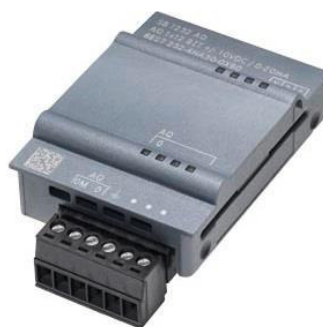
Figura 3.83. Signal Board SB1232.
