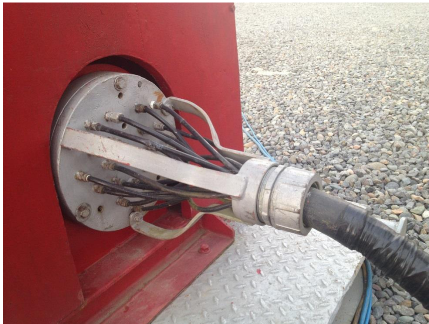
Figura 2.19. Conector circular del control remoto original CPV-23.
