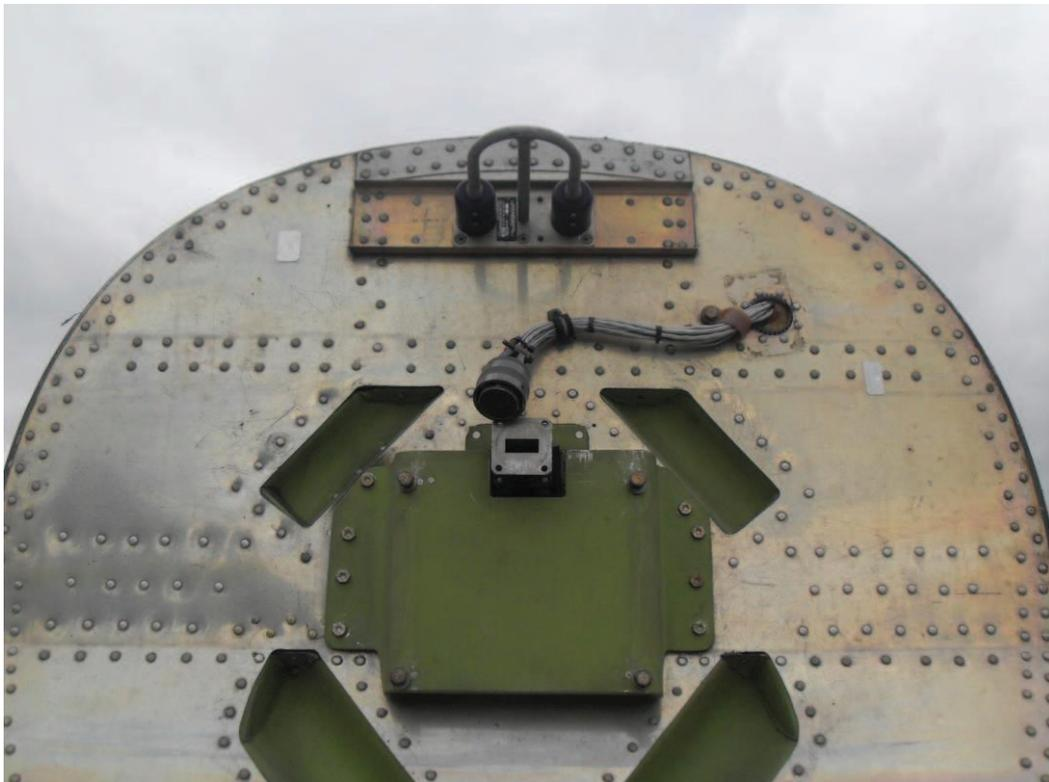
**Figura 3.12:** Antena glide slope
