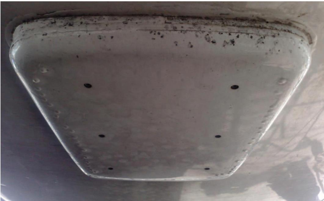
**Figura 3.21:** Antena loop ADF instalada
