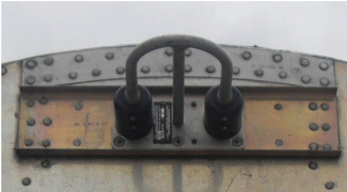
**Figura 3.23:** Antena glide slope instalada
