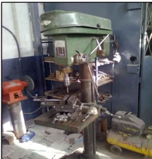
Figura 2.18 Taladro Morgan, modelo mfgtm54 20mm, 550w, 110v.
