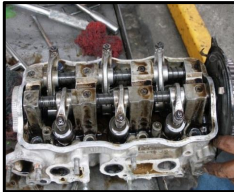
Figura 2.8: Culata Suzuki G10.
