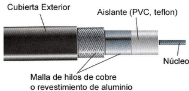
**Figura 4 Cable coaxial**
