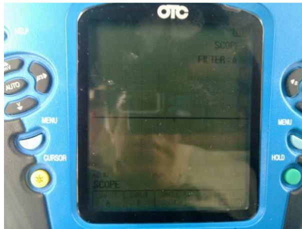
Gráfico No. 4.4: Corte a masa CAN LOW.
