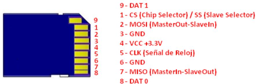
**Figura 111 Pinout Tarjeta SD**
