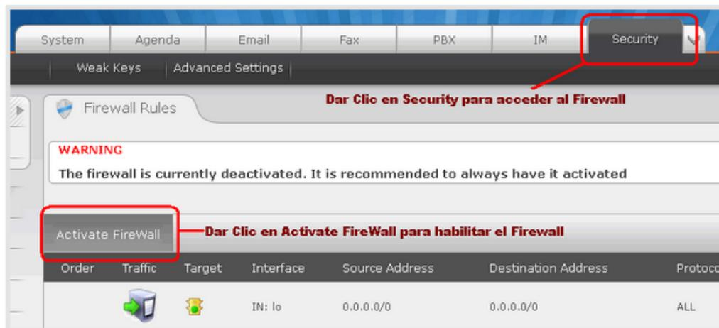
**FIGURA 6: FIREWALL ELASTIX**
