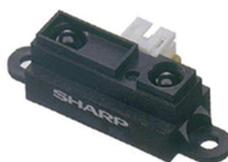
**Figura 3.28 Sensor SHARP GP2Y0A41SK0F<sup>70</sup>**
