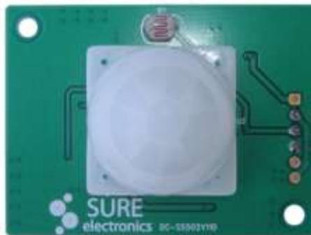
**Figura 14. Sensor PIR DC-SS502V110**
