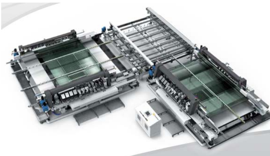
Figura 27. Pulidora bilateral Glaston Bavelloni XtraEdge 8.
