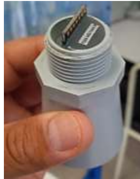
Figura 3. 21. Sensor HRXL- MAXSONAR-WRM (MB7369)
