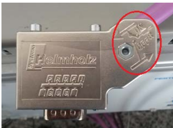
Figura 3.26: Selector de modo ON/OFF del conector Profibus
