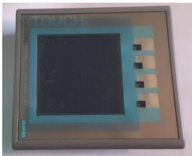
Figura 2.9. Panel SIMATIC HMI KTP400 BASIC MONOCROMÁTICO
