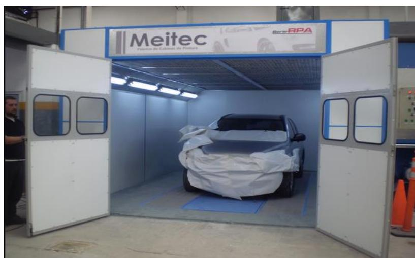
**Figura 5 Cabinas-horno**
