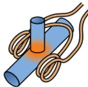
**Figura 13: Bobina helicoidal dividida**
