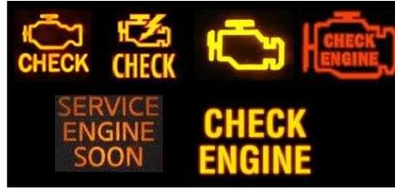
Figura 9. Lámpara MIL (Check Engine)
