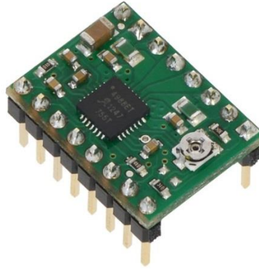
Figura 4.5: Driver motor a paso A4988. (Pololu, 2015)
