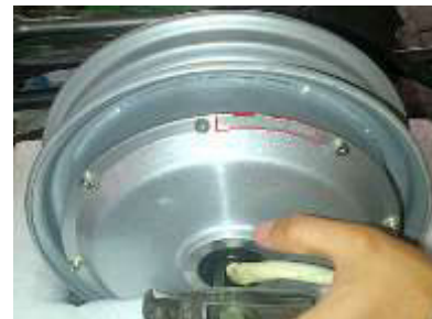
Fig. 5. Motor brushless 48V/4000W MOD-0704509598
