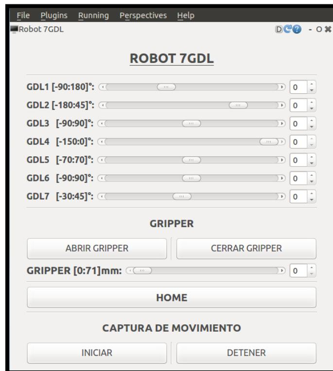
**Figura 109 GUI control robot 7GDL**
