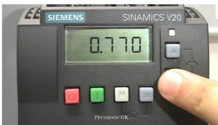
**Figura.68: BOP (Basic Operator Panel)**
