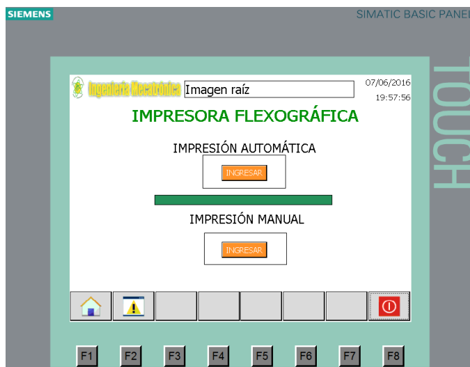
Figura 56: Ventana principal HMI
