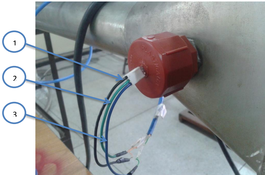
1.Cable Negro "GND"; 2.Cable Verde "Vout"; 3.Cable Azul "Vcc"
