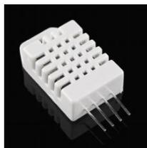
**Figura 24. Sensor AM2302/DHT22**
