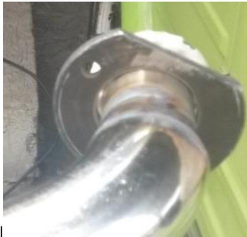
**Figura 37 Soporte principal del colector**
