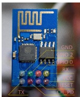
**Figura 14. ESP8266 ESP-01.**
