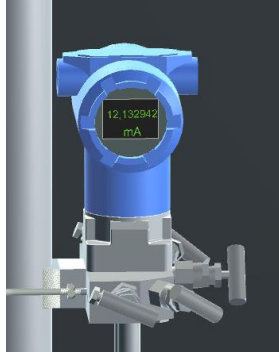
(c) Results presentation of an output corresponding to 12.1mA. Fig. 12. Transmitter changes to different current input values
