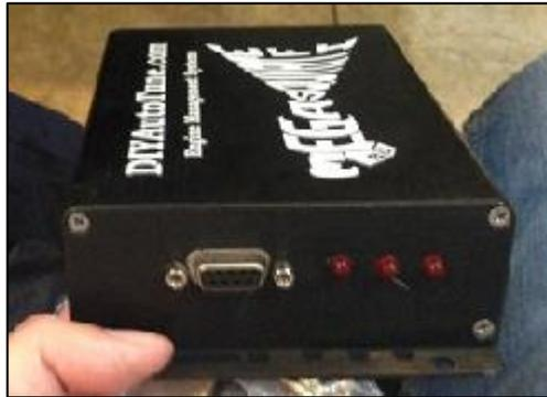
**Figura 38. Conector Serial DB9 MegaSquirt-II**
