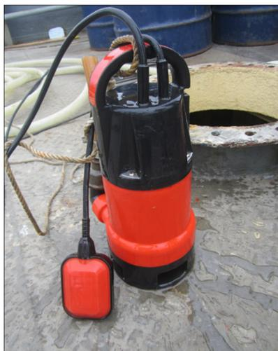
**Figura 2.16.** Bomba sumergible
