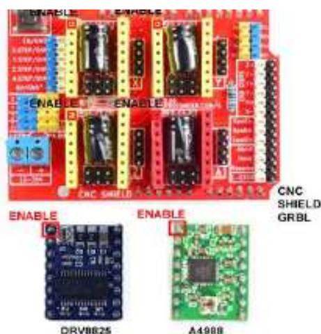
Figura 47. Modulo CNC shield y driver A4988
