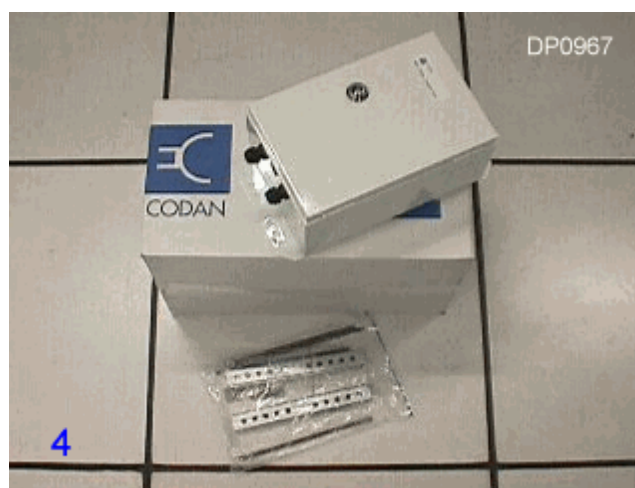
Figura. 2.69. (DP0967) Inner Box 5581 Main Power Supply
