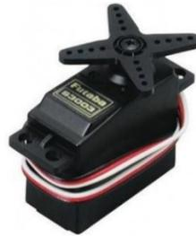
*Figura 49. Servomotor.*
