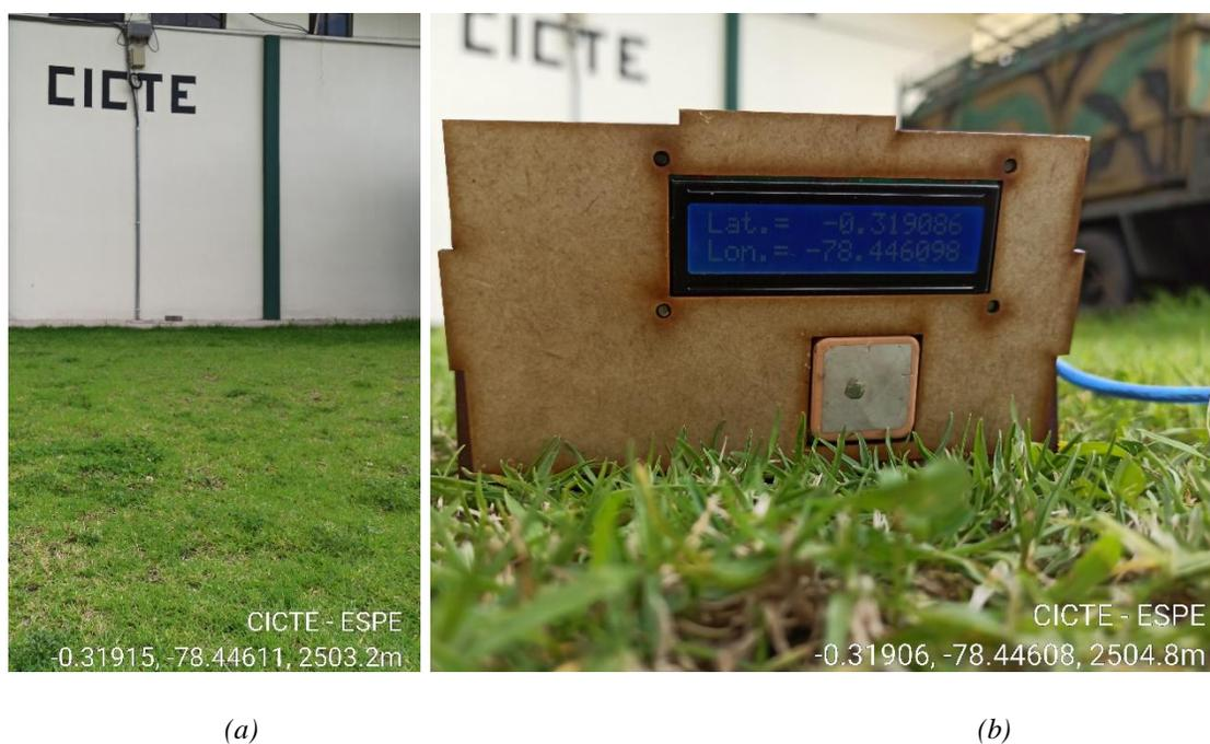
**Figura 22.** Coordenadas CICTE: (a) Open Camera (b) GPS u-Block NEO-6M
