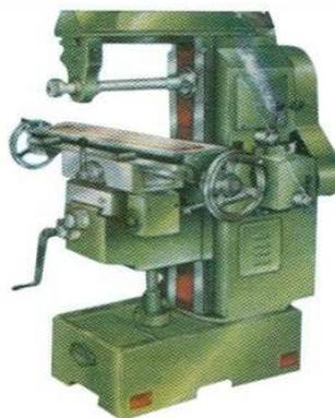
Fig. 1.1: Fresadora Horizontal <sup>1</sup>
