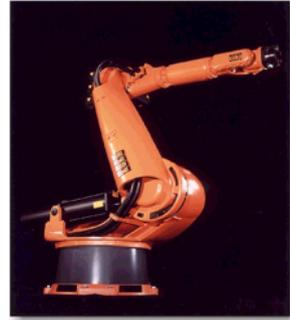
**Figura. 1.32. Robot art. Vertical (R)**
