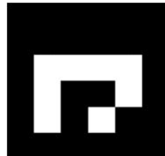
Figure 3. Pattern provided by the Aruco bookstore, necessary for the rotation and objective translation matrices of the UAV.
