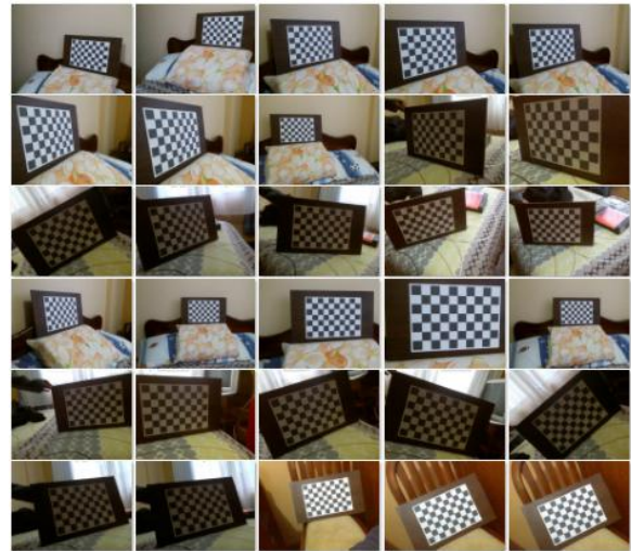
Figure 4. Photographs taken with the drone dj Tello to obtain the intrinsic and extrinsic parameters of the camera.
