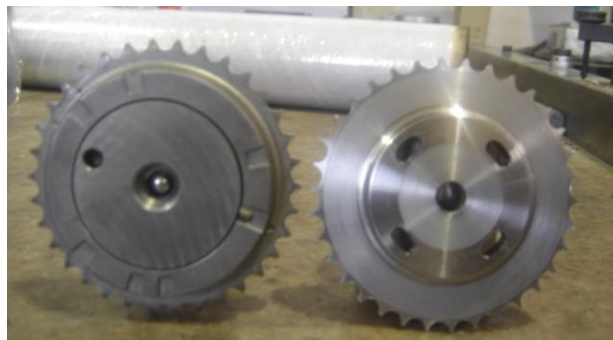
Figura 5.72: (Piñón original y piñón regulable)
