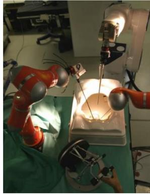
*Nota:* Dos robots KUKA LWR IV (robots naranjas), Stäubli RX90 (robot blanco) con endoscopio adjunto. Tomado de An Intelligent and Autonomous Endoscopic Guidance System for Minimally Invasive Surgery (P. 5763), por Weede et al., 2011, 2011 IEEE International Conference on Robotics and Automation.
