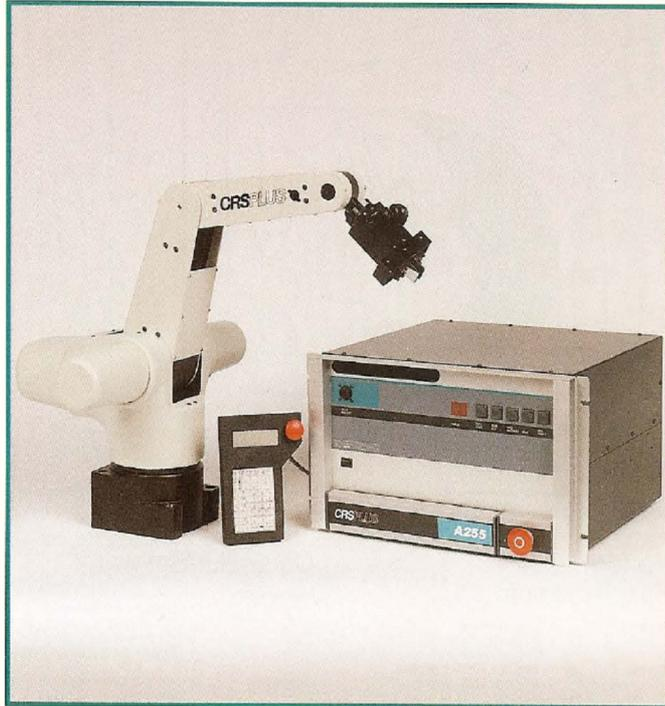
The A255 Robot is designed to work with a wide variety of peripherals including rotary tables, bowl feeders, conveyor belts, host computers, vision systems and other advanced sensors.
