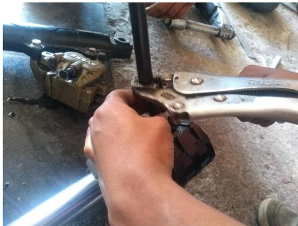
**Figura 58***Mordaza Delantera y Bomba de Freno*
