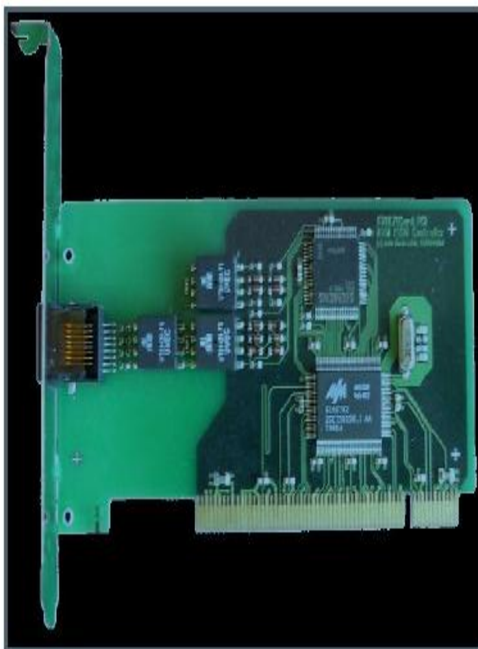
Figura 2. 8. Tarjeta ISDN AVM FRITZ 1 puerto
