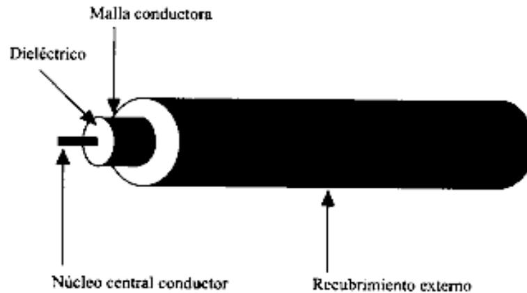
**Figura 3.14. Cable coaxial**
