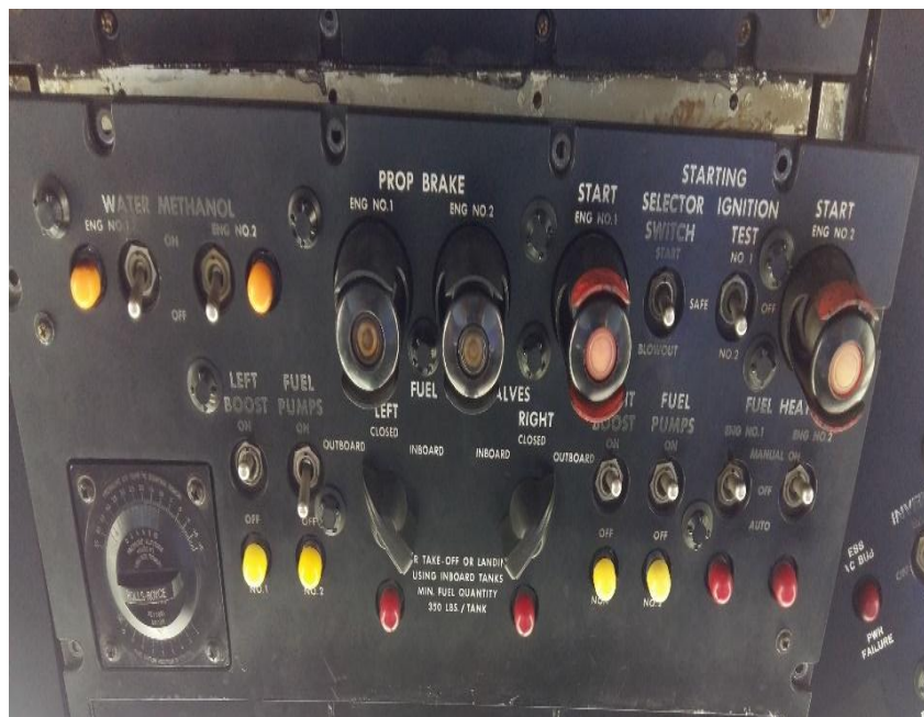
Figura 12 Starting Selector Switch Engine N° 1
