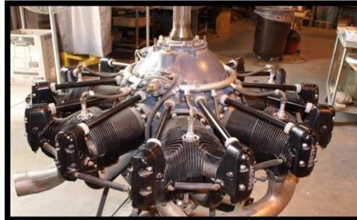
**FIGURA 4 Motor Radial Jacobs R755**
