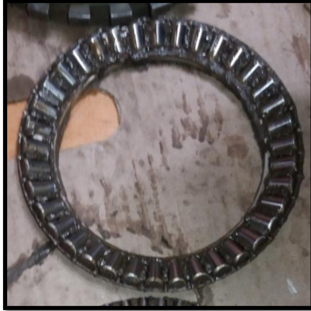
Figura 57: Cage assembly, centrifugal and rollers
