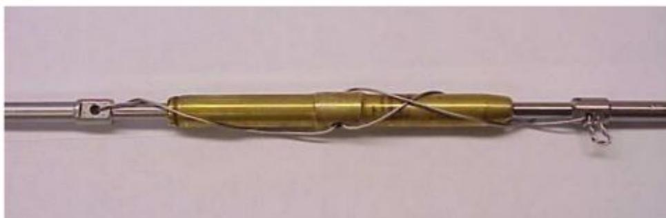
**Figura 15** Turnbuckle
