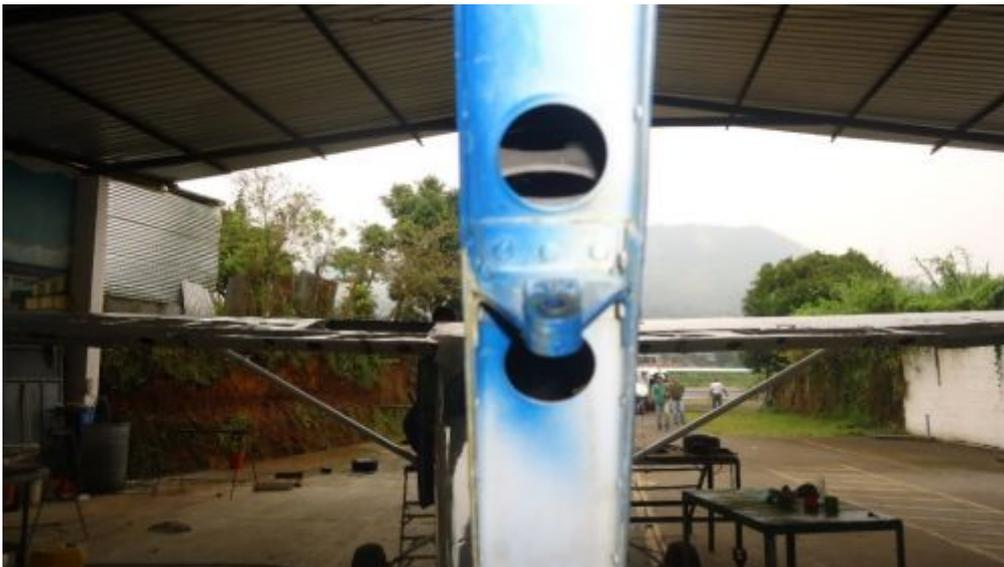
**Figura 26** Bisagra de rudder intermedia
