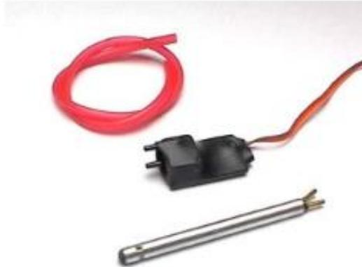
The optional *Airspeed Sensor* consists of a pitot tube and a precision, differential pressure sensor. By sampling the ambient air temperature, the current flight speed of the model is calculated by the ECU, from the measured difference in static versus dynamic pressure.
